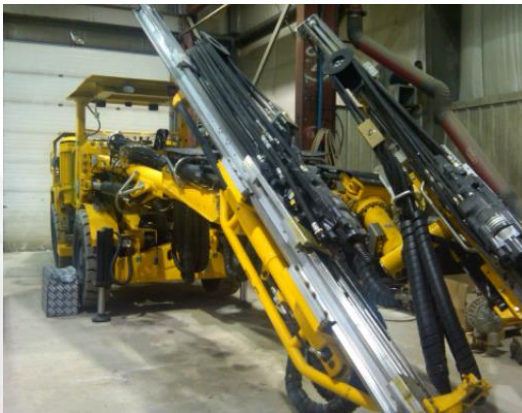
2-Boom Jumbo Drill BUCKO LAKE MINE
